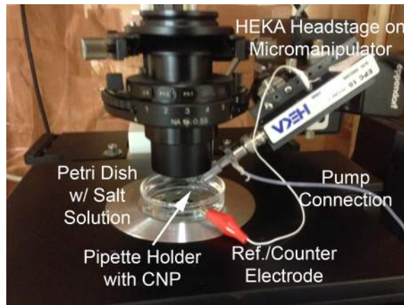
Figure 41. Capacitance characterization setup. A CNP is mounted on a HEKA headstage which is mounted on a micromanipulator which is mounted on an inverted microscope. The pipette coupling is connected to a microinjection pump and the ground is connected to a reference/counter electrode in solution. The CNP tip is immersed in a petri dish filled with PBS or other simple salt solution such as KCl.
